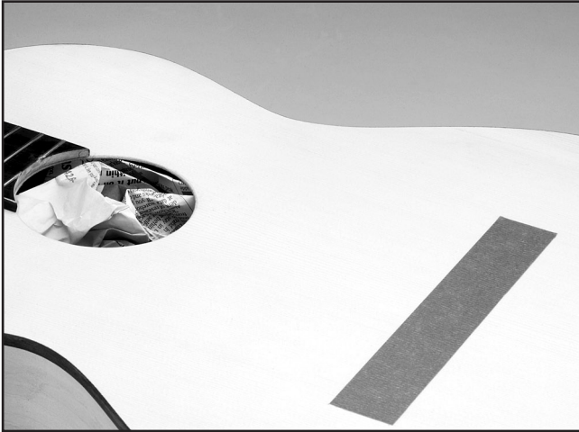
Figure 8. Masked bridge area and blocked sound hole.
